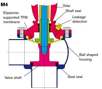
DELTA M4 valves feature an elastomer supported flat TFM membrane. Suitable for most applications.
