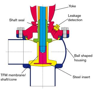
DELTA MP4 valves feature a TFM membrane, shaft & seat all in one piece. Especially suitable for applications where additional elastomer seals are not allowed or are incompatible.
