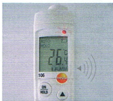
Audible and optical alarm (LED lights up)
