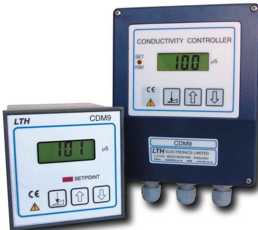
The CDM9 Conductivity indicator controller is available as either a panel or surface mounting version in an IP66 enclosure with a 3½ digit liquid crystal display.
