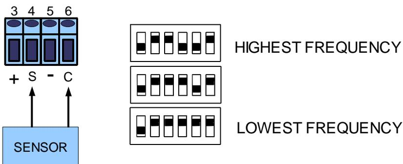
**NOTE: If the cable to the coil is shielded, connect the shield to “-” (terminal 5) ONLY. Do not connect the shield to anything at the other (coil) end of the cable. The shield has to be isolated from earth ground and all other equipment or electrical connections.**
