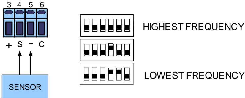
5.1.1.5. NAMUR Sensors, Data Industrial Two Wire Flow Meters
