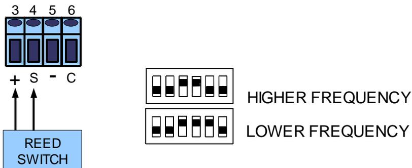
**NOTE: Different reed switches and dry contacts have different bouncing time. Test and evaluate carefully to determine the right DIP switch setting.**
