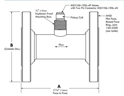
Meter size based on normal inside diameter of pipe.
